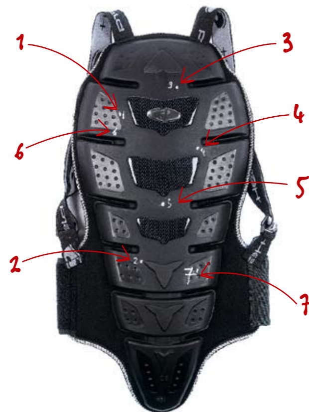
The impact zones: Strikes 1-5 are at spots used by the European standard. Impacts six and seven varied by protector, depending on where the tester, Dr Roderick Woods, assessed a zone that was potentially weaker than the rest.
